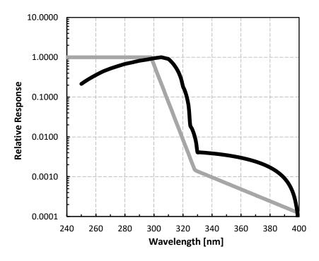
Spectral response estimate of Apogee SU-300 UV-I/UV-B sensors. Spectral response was modeled from sensitivity of the photodetector and transmittance of the diffuser. Gray line is the Erythemal Action Spectrum and provides a relative indication of skin damage caused by UV radiation.
