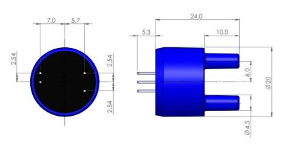
NOTE: 4.5mm OD push-fit tubing connectors.
