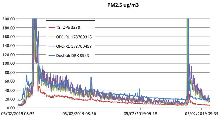
Figure 2 shows a comparison of PM2.5 monitoring by an OPC-R series sensor and TSI OPS 3330 and DustTrak instruments. All are set at 5s averaging and are sampling the ambient air of a work shop, the raw 3330 data has been used to calculate a PM figure.
