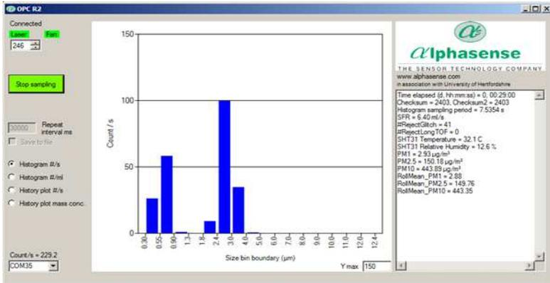
Figure 1 shows the OPC-R2 particle size distribution for the test aerosol.
