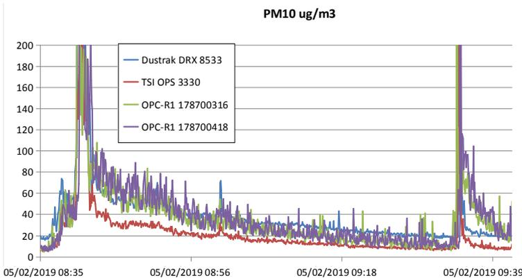
Figure 3 shows a comparison of PM10 monitoring by an OPC-R series sensor and TSI OPS 3330 and DustTrak instruments.
