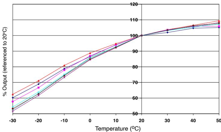
Figure 1 shows the temperature dependence of sensitivity at 2ppm NO.
