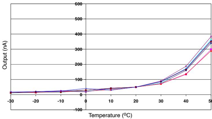
Figure 2 shows the variation in zero output of the working electrode caused by changes in temperature, expressed as nA.
