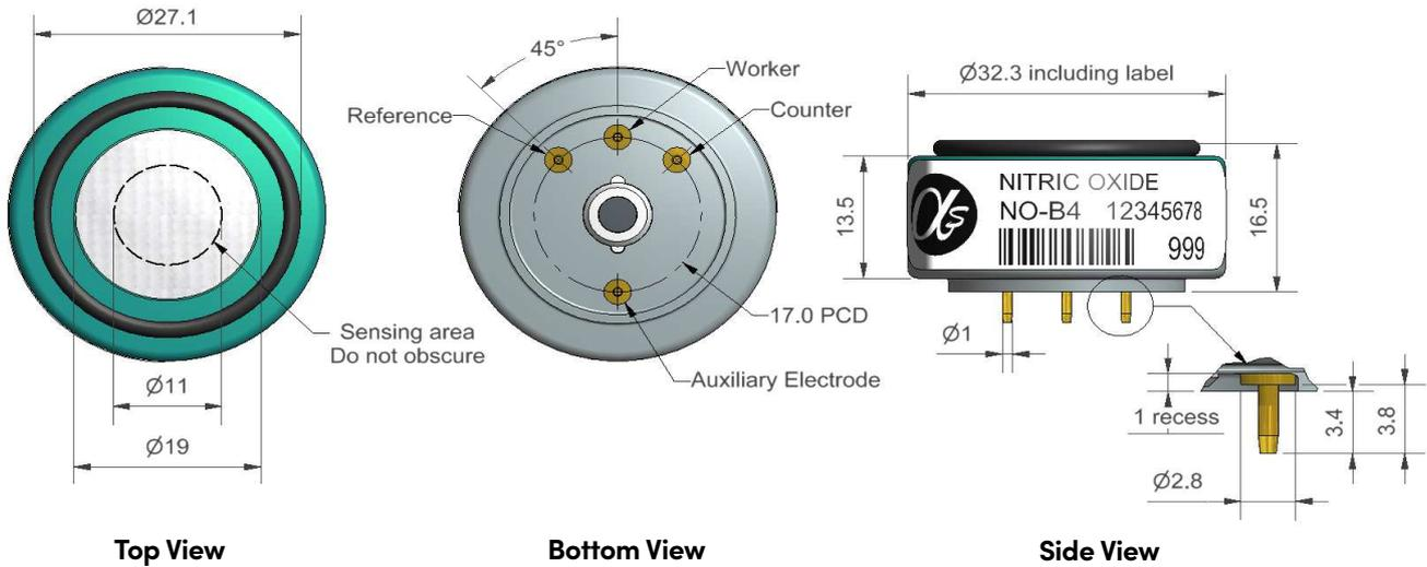
Dimensions are in millimetres ( $\pm 0.1$  mm).
