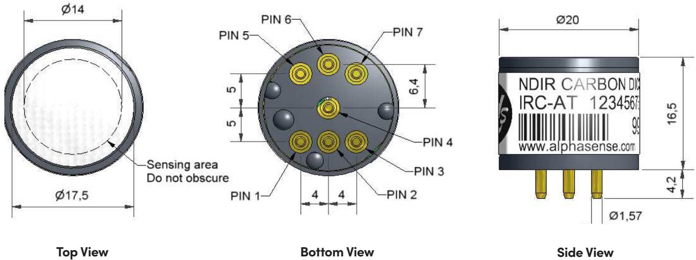
Dimensions are in millimetres ( $\pm 0.15$ mm).
