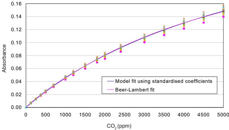
Typical response from 0 to 5000ppm CO<sub>2</sub>.
