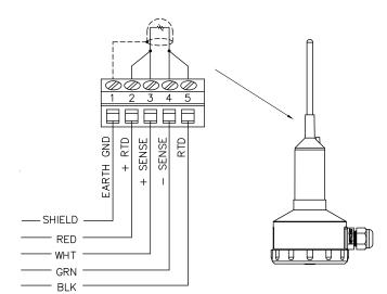
NOTE: The terminal marked "EARTH GND" should be connected to properly grounded tower, or grounding conductor, as close to the sensor as possible. Failure to do so may result in damage due to static discharge.
